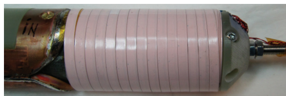
The world's highest field superconducting magnet is made out of \text{YBa}_2\text{Cu}_3\text{O}_{7-x} tape. It generated 4 Tesla in a 31 Tesla background field at the NHMFL.
