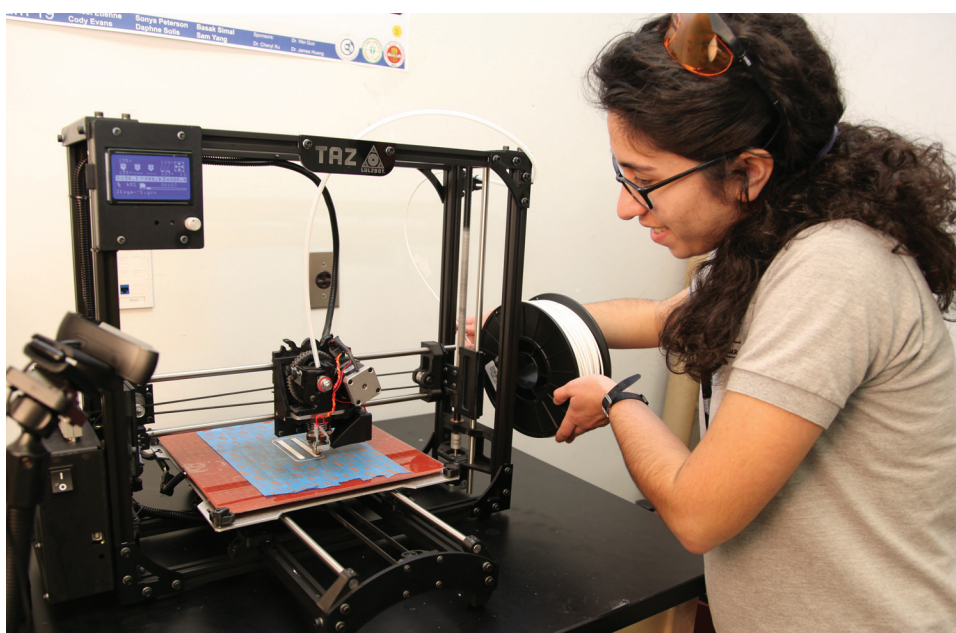
This additive manufacturing testbed in Dr. Cheryl Xu's lab is capable of manufacturing freeform shapes and controlling microstructure and properties for metal, ceramics, or metal-ceramics joining structures.
