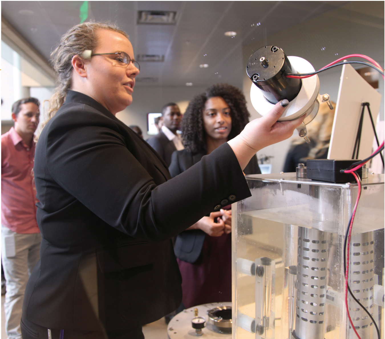
At Senior Design Day, a senior ME student assembles a working prototype of a magnetically coupled pump system for a project sponsored by the Florida Space Grant Consortium and NASA Marshall Space Flight Center. The pump is designed to mix cryogenic fluids in a space vehicle's cryogenic tank without adding heat to the system.
