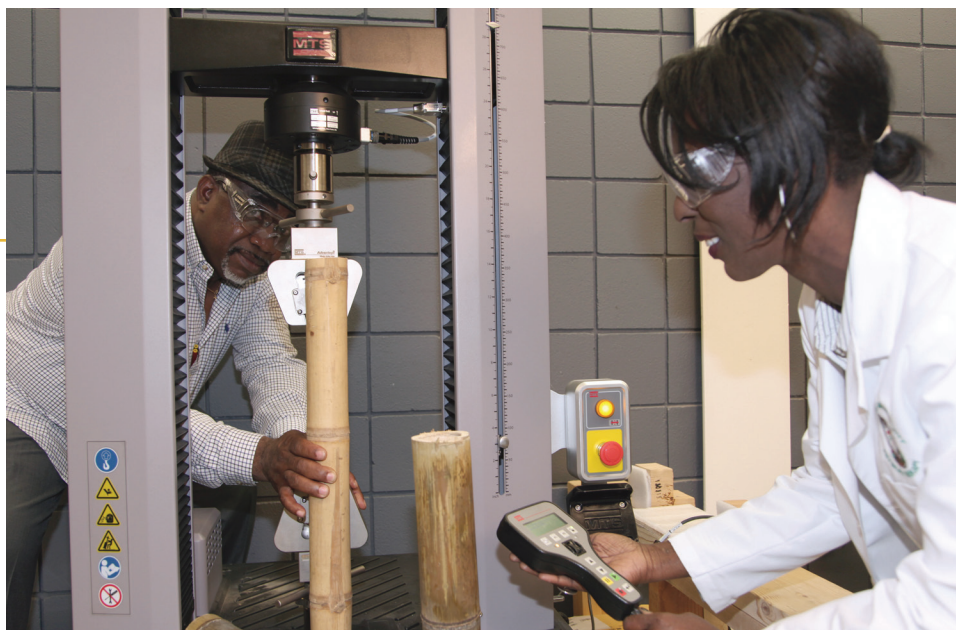
Dr. Peter N. Kalu and Dr. Kischa S. Reed (FAMU Allied Health) testing bamboo for its mechanical properties for exoskeleton design and manufacturing.
