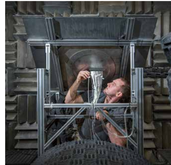
The anechoic test chamber at the Florida Center for Advanced Aero-Propulsion.
